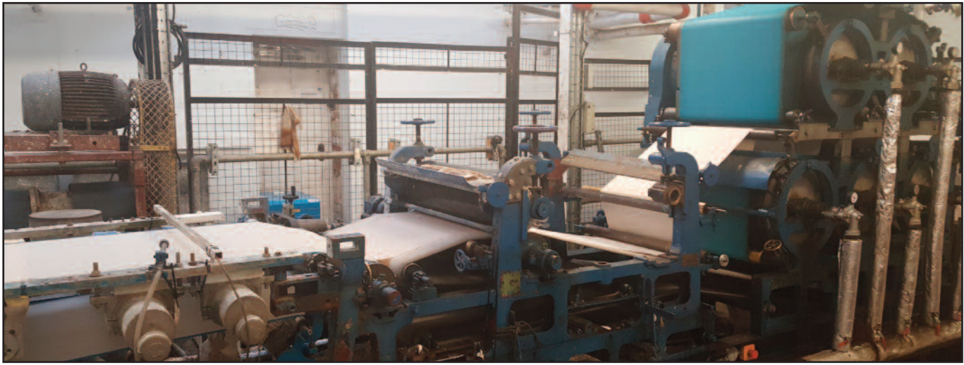
The 1902 Fourdrinier conveyor mould paper machine will soon be partnered with a cylinder mould paper machine
